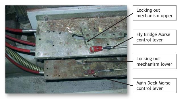
Change-Over Mechanism from upper deck to lower deck, which is situated below lower deck level was visually tested under operation. All linkages were suitably lubricated and in good working order.
