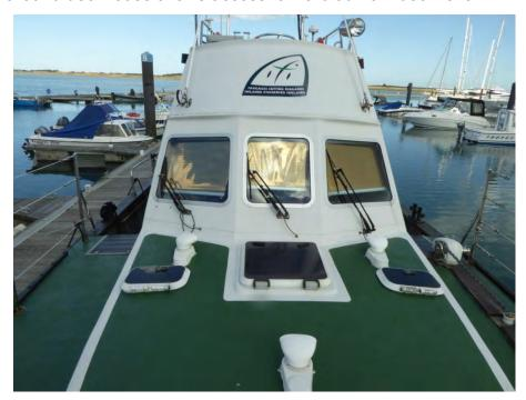
The main deck is flush over the engineroom whih a raised coaming to provide access and limited headroom. A cradle is provided for an inflatable dinghy. A folding hydraulic crane is used to launch and recover the dinghy or other equipment stored on deck
