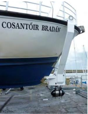
The walk-around deckhouse allows access forward at main deck level. A hydraulic gantry is mounted forward and used to deploy underwater equipment as shown below. The main deck is raised in way of the engineroom and provides a moulded cradle for an inflatable dinghy. A folding hydraulic crane is used to launch and recover the dinghy or other equipment stored on deck.
