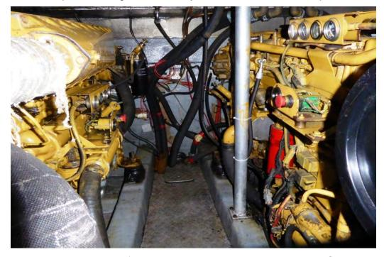
Two silenced generators are fitted in the engineroom. These Panda Compact Power units provide 220 V AC for domestic and research equipment separately. A Victron Energy multiplus Compact is fitted to provide a charge management system for a number of battery banks and to use 24V DC to provide a 220volt AC output.
