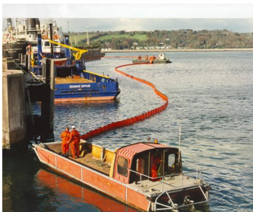
Deploying a boom for pollution control
