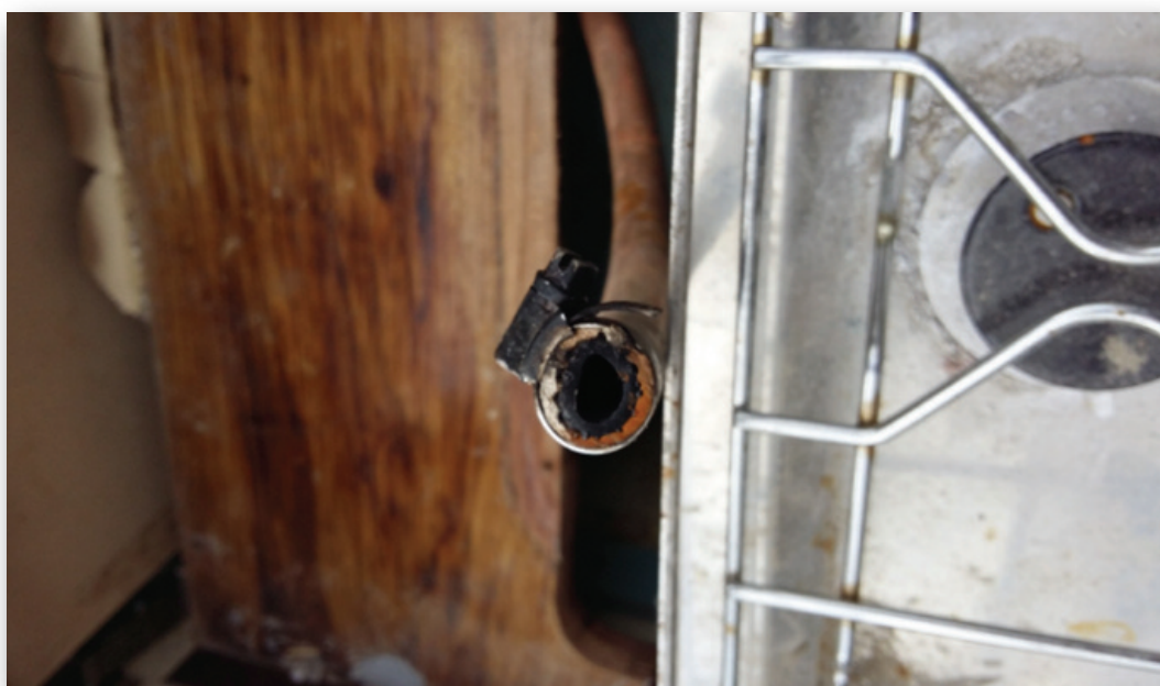
Photograph No.5 - Gas hose cooker end as found, charred and distorted.
