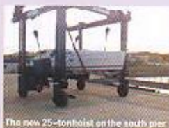
The new 25-ton hoist on the south pier
